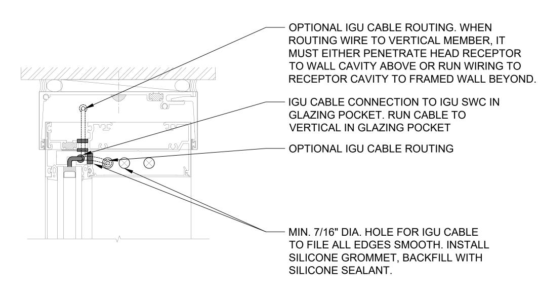
**INSTALLER TO PROVIDE GROMMETS** AT ALL FRAME PENETRATIONS WHERE POSSIBLE TO AVOID CABLE DAMAGE.
